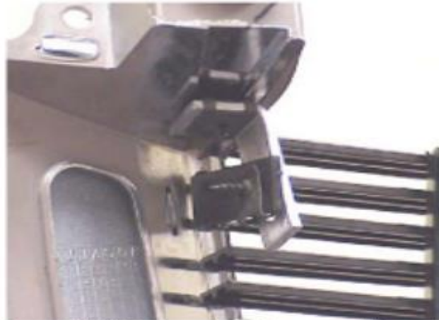
(Photo #2) Note location of upper side mount
