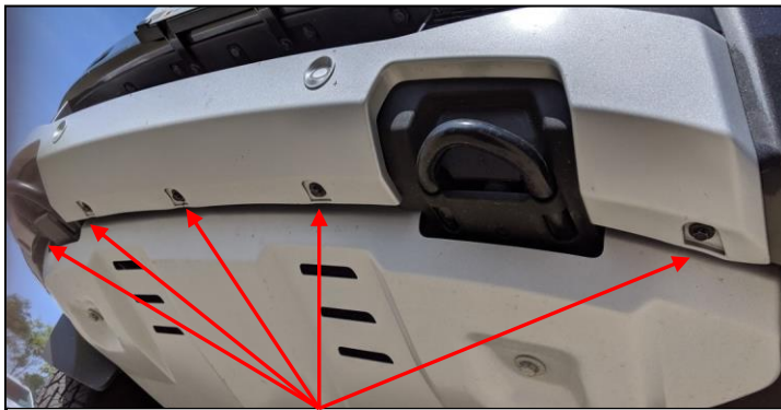
(Fig 1) Five Lower Valance Bolts
