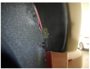
**STEP 10:** To secure the front slot in the Fender Flare to the body, take the black metal clip and slide it over the Fender Flare and the inner wheel arch lip. Position the clip so that the barb in the clip locates in the slot of the Fender Flare. Ensure all fixing points are tight and secure and that the rubber seal is flush neatly against the vehicle body.
