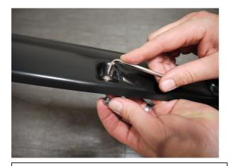
**STEP 1:** Attach the 10 bolts and nuts to each Fender Flare using a 3/16" Allen key and a 1/2" wrench/socket. wrench/socket. (wrench /socket and Allen key not supplied). Ensure inside of Fender Flares where the rubber seal is attached is clean, using the alcohol wipes provided. Wipe away any residue with a dry clean cloth.
