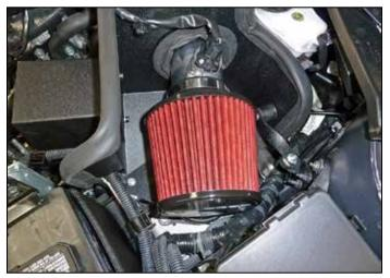
14. Place the Spectre<sup>®</sup> high flow air cleaner onto intake tube making sure calibration sleeve is located properly and tighten clamp.
