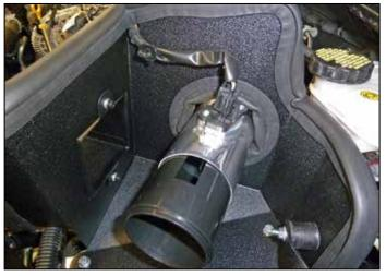
12. Push the Spectre<sup>®</sup> air intake tube through the right side of the heatshield and into coupler on throttle housing and tighten hose clamp. Install MAF sensor into intake tube with the two 4mm screws provided, then route MAF connector wiring through slot in heatshield under edge trim. Slide MAF calibration sleeve into intake tube. **NOTE: Calibration sleeve must be installed or vehicle will not perform properly and warranty will be voided.**
