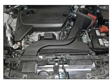
15. Install air intake duct removed in step 4.
