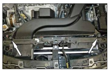
4. Remove the two bolts securing air intake duct and remove duct. This will be reinstalled in a later step.
