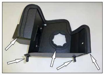
9. Install edge trim onto heatshield as shown and trim to fit. Install the two nylon mounts with provided hardware as shown.
