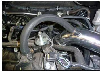
13. Install PCV hose onto intake tube and valve cover, secure with provided clamps.
