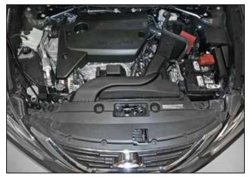
16. Install radiator cover removed in step 3.
