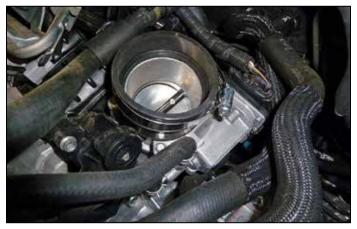
8. Install the Spectre<sup>®</sup> reducer coupler onto throttle housing and secure with provided clamp.
