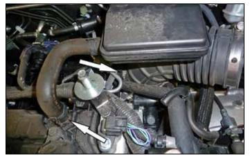
7. Release spring clamp and remove PCV hose from valve cover, then loosen hose clamp on intake boot and remove boot.
