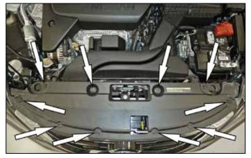
3. Remove the eight plastic clips securing radiator cover by lifting center of clip. After removing all clips lift cover off. Save for a later step
