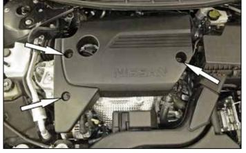
2. Remove the three bolts securing engine cover and remove cover.
