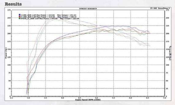
The graph above shows that the MMINT-GEN4-10 base kit (in red) gained 3whp and 4.5wtq over the stock intercooler setup (in green). The MMINT-GEN4-10R race kit (in blue) performed even better, gaining 12whp and 8wtq over the stock setup.
