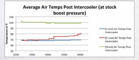
The graph above is comparing the average air intake temperatures after the air has passed through the intercooler. The MMINT-GEN4-10 (Z-Line) unit cooled the air about 23°F better than the stock unit, and the MMINT-GEN4-10R (J-Line) cooled the air about 28°F better than
