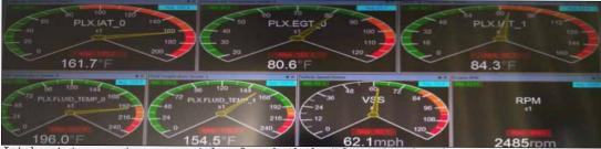
Intake air temperatures were taken from both the inlet and outlet of intercoolers using PLX K-type thermocouples. Boost pressure was also tested to ensure that no dramatic pressure drop occurs due to the larger Mishimoto intercooler.
