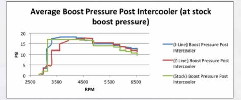
The graph above shows the boost pressure after the air has gone through the intercooler. Both Mishimoto units gained almost a full pound of pressure over the stock unit. This improvement is due to the flow patterns that were carefully engineered by Mishimoto using CFD software.
