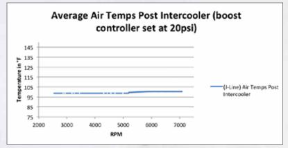
The graph above shows that the J-Line's outlet air temperature was still reaching near ambient temp, though it did rise slightly due to the added boost pressure.
