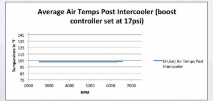
The graph above shows that the J-Line's outlet air temperature was almost reaching ambient temp.
