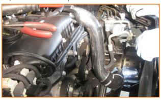
5. Install T-Bolts clamps onto cold side piping.
