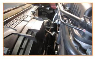
12. Remove (2) 10mm bolts for the A/C condenser.
