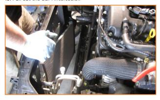
20. Remove (2) 10mm bolts for the Airflow sensor.
