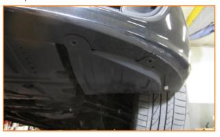
**4.** Remove the (4) plastic screws for the intake dam. Lift up and remove from vehicle.
