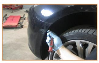
**6.** Remove the (8) plastic screws for the front bumper on the radiator support.
