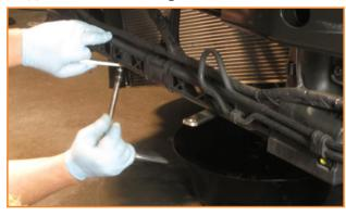
2. Mount the intercooler, tighten M6 x 1.0 bolts, and install the intercooler with the provided (2) M12 x 1.75 x 20mm bolts. Leave loose. Install Mishimoto couplers onto intercooler.
