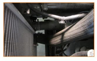
**16.** Remove (4) 10mm bolts holding the radiator to the intercooler. (2 on each side of the radiator)
