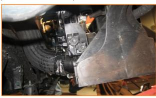
17. Pull up on A/C condenser to remove from the radiator holsters and remove radiator from the vehicle. Do not remove the A/C condenser from the vehicle, as this will require you to recharge the A/C system once completed.
