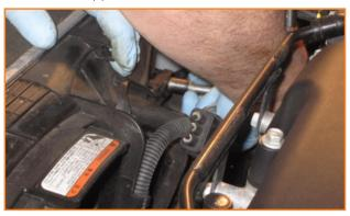
14. Plug fan in and reattach wiring harness onto the fan shroud and reinstall the coolant overflow container and overflow rubber line.
