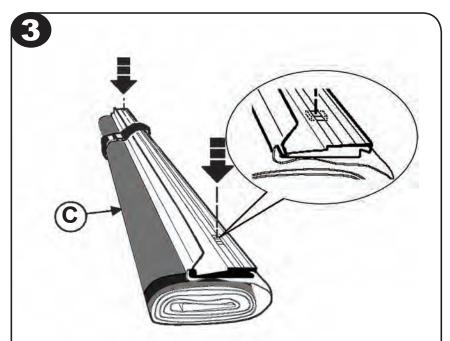
Cover is shipped in preassembled rolled open position. The visible bar (with nuts in channel) goes to front behind cab.
