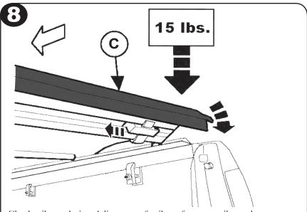
Check tailgate closing. Adjust rear of rails up for more tailgate clearance, or down for less clearance. Check cover tension with tailgate down. Closing bar down and latching should take about 15 lbs. of pressure.
