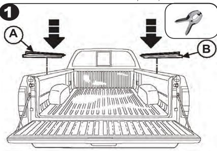
**Driver Side** - end of rail with slotted hole goes to front behind cab, trigger latch to rear.
