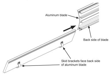
E. Locate factory marks on back of blade. Place slide hinge on blade as shown and align both lower holes with marks on blade.
