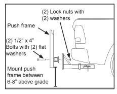
**NOTE**: In some cases, clearance under receiver may be less than 6". If so, plow will still operate properly, but ground clearance will be limited. Use care on uneven surfaces.
