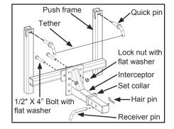
E. Push set collar tight against receiver, hold and tighten set screw with 3/16" hex wrench.
