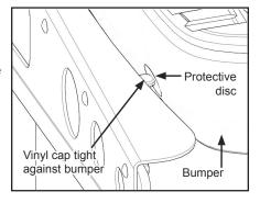
**TIP:** If clamp assembly butts up to receiver before both bumper caps are against bumper, remove clamp and reassemble on ball mount side of frame.
