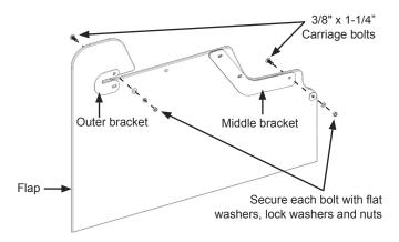
C. Align holes in brackets and flap then secure to frame with carriage bolts, large flat washers, lock washers and nuts. Use 3/8" x 1-1/2" carriage bolts when bolting through frame, flap and brackets. Use 3/8" x 1-1/4" carriage bolts when bolting through frame and flap. Tighten nuts until lock washers are fully compressed.
