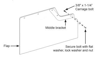
B. Align holes in bracket and flap then secure to frame with carriage bolts, large flat washers, lock washers and nuts. Use 3/8" x 1-1/2" carriage bolts when bolting through frame, flap and middle bracket. Use 3/8" x 1-1/4" carriage bolts when bolting through frame and flap. Tighten nuts until lock washers are fully compressed.
