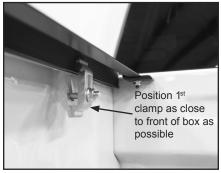
**NOTE:** Images below illustrate clamping options. **Option A** depicts standard clamping orientation lower on the side rail. **Option B** depicts alternate clamping orientation with half of clamp assembly rotated 180° to provide better grip at top of side rail.
