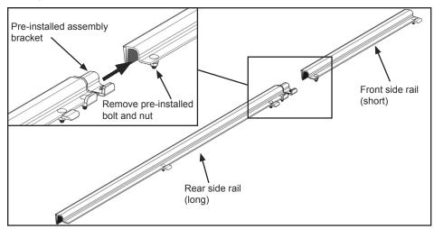
D. Attach short side rail (front) to assembly bracket with previously removed 1/4"-20 x 3/4" carriage bolt and 1/4"-20 nylock hex nut. Align side rails then tighten with 7/16" wrench.
