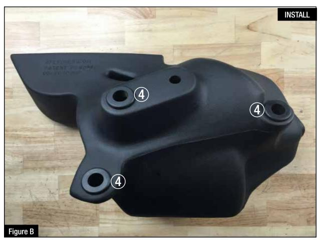
**Refer to Figure B for step 5** Step 5. Install the 3 provided rubber grommets (4) on the bottom of the aFe air box as shown.
