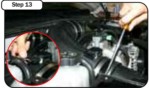
Tighten all clamps with 5/16" nut driver. Re-connect MAF sensor harness.
