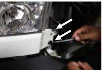
Locate the two trim pins on the lower headlight trim panel and remove the two pins
