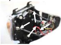
Connect the power source and each of the three light bulb harnesse into the Anzo headlights
