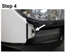
Remove the 10mm screw located at the bottom of the headlight housing
