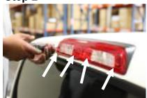
Remove the four phillips screws on the third brake light housing
