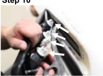
Remove the third brake light by disconnecting the power source and the three light bulb harnesses
