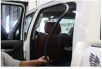
Remove the rubber molding surrounding the rear door frame
