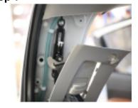
Remove the upper inner lining panel
