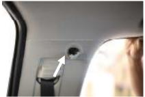
Open the cap directly above the sea belt holster to separate the inner lining panel
