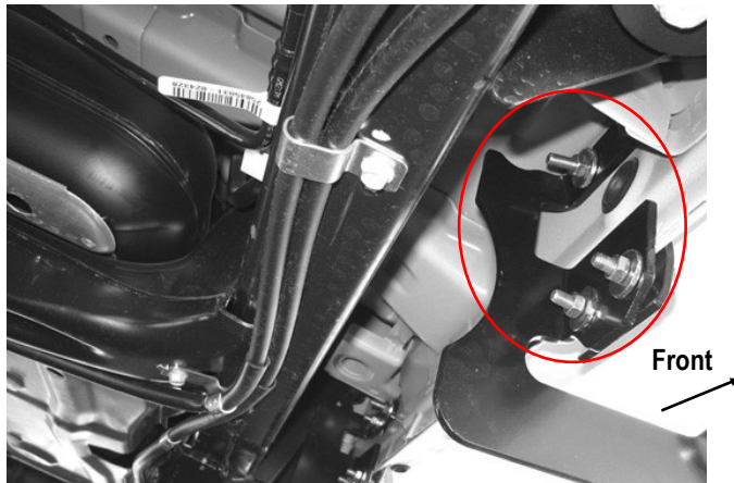
(Fig 6) Driver Side Center Mounting Bracket Installation
