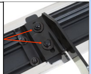
(Fig 6) Step Bar Installed on Bracket Installed (Example)
