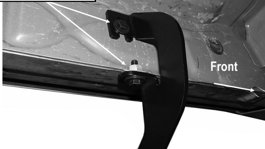
(Fig 6) Driver Front Mounting Bracket Installed
