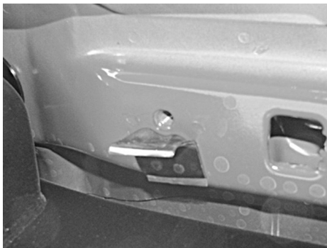
(Fig 2) Vehicle with 8mm Threaded Hole In Floor Panel
