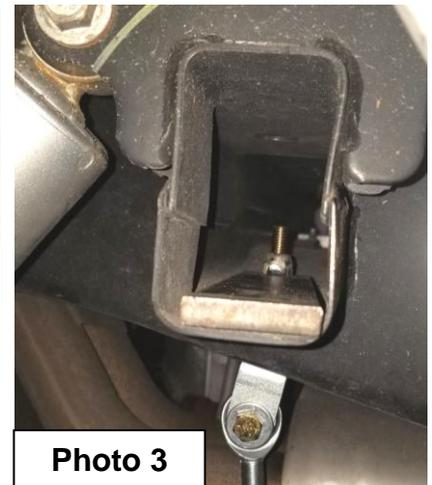
6. Slide the supplied end link mounting bracket plate into the crossbeam far enough for the attached nut to align with the newly drilled hole. The plate labelled 6447-050 is used on the drivers side while 6447-051 is used on the passenger side. The mounting processes are the same on both sides. (**Photo 3 & 4**)
