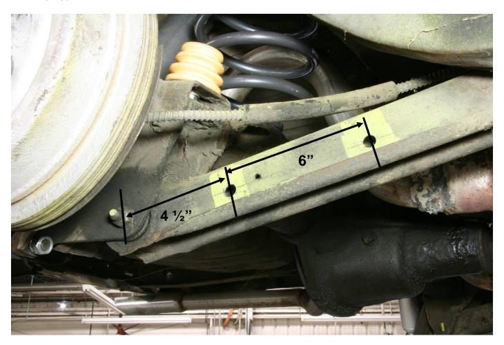
7. Position a spacer tube behind each hole in the control arm. Make sure a 1/2-inch bolt is able to go into each hole and spacer tube. Use the 1/2-inch bolts, Nyloc nuts, and washers to fasten the Anti-Sway Bars to the control arm. Tighten to approximately 80ft/lbs of torque.
