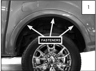
Remove (3) factory installed plastic fasteners from the driver side rear wheel well using a phillips screwdriver. Needle nose pliers may be needed to extract the fasteners.
