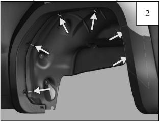
While holding the rear flare in place, mark the flare's (6) hole locations using a grease pencil.
