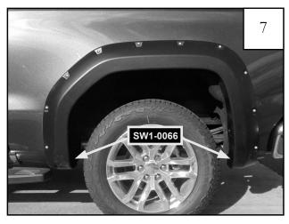
Using an electric drill/driver, install rear flare using (2) SW1-0066 drill screws through the sheet metal flanges at the bottom of the fender.
