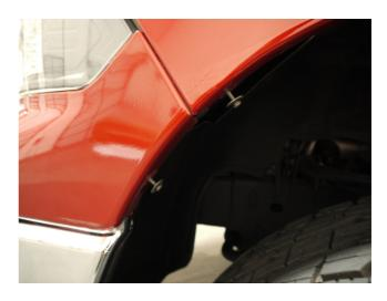
**STEP 2:** Remove all factory bolts and retain for installation of Fender Flares.
