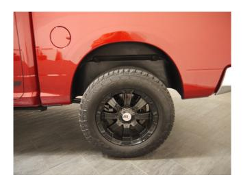
**STEP 6:** Clean the body areas where the Fender Flares will makes contact. Use the supplied alcohol wipe.
