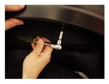
STEP 4: Reattach all bolts removed in step 2.
