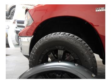
**STEP 1:** Clean the body areas where the Fender Flares will makes contact. Use the supplied alcohol wipe.
