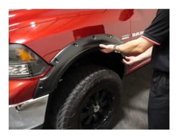
**STEP 3:** Place the Fender Flare onto the vehicle and fit into the correct position following the contours of the body.
