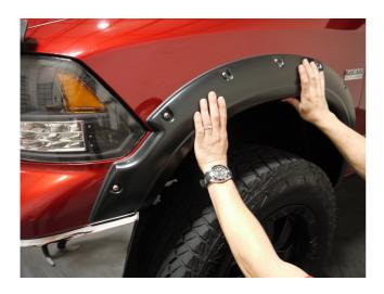
**STEP 5:** Check fitment and contour of Fender Flare to headlight housing and readjust if necessary.
