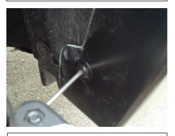
STEP 5: Reinstall the #15 Torx head screw.
