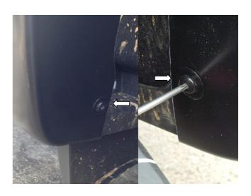
STEP 10: Reinstall the #15Torx head screws.
