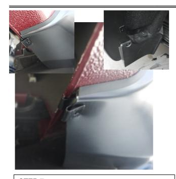
**STEP 7:** Slide the top edge of rear front mudguard cut out behind the factory mudguard. Install the E shape clip so that the clip slides over the inner sheet metal lip and is in line with the slot in the underside of Fender Flare. To secure the clip to Fender Flare apply inward tension on Fender Flare to the vehicle fender when installing the E clip, position the clip so that the barb in the clip locates in the slot of the Fender Flare.
