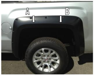
**STEP 12:** To secure the Fender Flare to vehicle body, ensure Fender Flare is in position of best fit and the slots in position **A** and **B** (Step: 11) are over the vacant holes in the wheel arch molding. Apply pressure on Fender Flare towards the vehicle fender when reinstalling the previously removed factory screws in position **A** and **B** using a #15 Torx head screwdriver.
