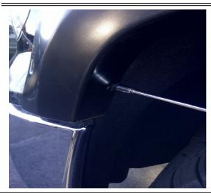
**STEP 7:** Loosely re-install factory screw through the remaining slot in the front upper wheel arch molding. Ensure Fender Flare is centered and in position of best fit on fender. Tighten all front fender fixing points to ensure a tight and secure fit and that the rubber seal is flush neatly against the vehicle body.
