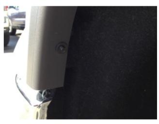
**STEP 4:** Using a 7mm or 8 mm socket, remove upper front wheel arch molding screw. Maintain screws for reinstall.
