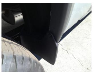
**STEP 10:** Using #15 Torx head screwdriver, remove upper screw as previously noted in position **C** from the factory mud flap deflector. Maintain screws for re-install.
