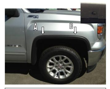
**STEP 2:** Place Fender Flare on the vehicle into the position of best fit. Note where (4) slots in Fender Flare correspond with (4) existing screws in the vehicle wheel arch molding. Remove Fender Flare. Remove the existing vehicle screws in location **A** and **B** using #15 Torx head screwdriver. Maintain screws for re-install.
