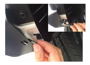
**STEP 14:** Remove remaining Hooked end Short Clip from hardware kit. Remove 10mm screw from previously noted area "**A**" in STEP 14 that aligns with mounting slot in Fender Flare. Install hook end of short clip into Fender Flare as shown above and re-install 10mm screw.
