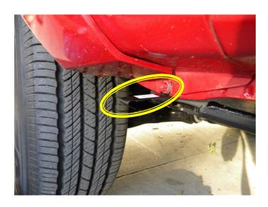
**STEP 5:** Remove Hooked end Long Clip from hardware kit and install in above shown orientation using the 10mm screw removed from the body sheet metal join in STEP 8 as Special Note area "**A**".
