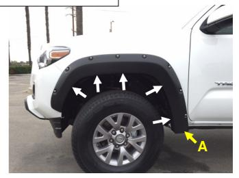
STEP 2: Hold Fender Flare on the vehicle in the position of best fit. For models <u>with</u> factory installed Fender Flares, note where above marked holes in Fender Flare align with existing screws in the vehicle. Make special note of "A". Remove the EGR Fender Flare and remove the (5) above indicated screws from the factory flare with a 10mm socket. <u>DO NOT</u> remove the factory flare, the EGR Fender Flare installs directly over the factory flare.
