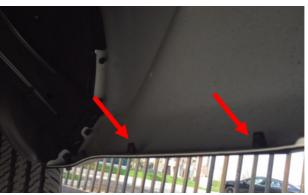
**IMPORTANT NOTE FOR REAR SPOILER FIN:** Using a 10mm socket, remove the (2) factory screws from the rear spoiler fin as shown. Pull (2) insert s out of vehicle body, spoiler fin has double sided tape adhered to the vehicle, pull off to remove spoiler fin from vehicle as shown. Surface area on vehicle where the double sided tape was adhered to on spoiler fin will need to be cleaned prior to Fender Flare install.
