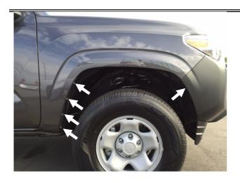
**STEP 3:** For models <u>without</u> factory installed Fender Flares, remove the (5) above indicated screws from the wheel liner with a 10mm socket and retain for later reinstallation.
