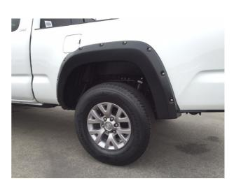
**STEP 15:** If necessary, make minor adjustments to the flares position to achieve the best fit for your vehicle and to ensure that the rubber seal is sitting flat against the painted vehicle surface. When satisfied fully tighten all screw locations, in the above order in which they were just installed. Repeat install for opposite side.
