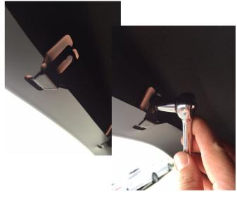
**STEP 7:** Ensure that the rubber seal is sitting flat against the painted vehicle surface, pay special attention to front area circled above. Using (3) previously removed 10mm screws from STEP 6 or 7, reinstall at above marked hole positions. Do not fully tighten screws at this stage.
