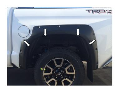
STEP 14: Install remaining short screws at the 4 fixing points located on image above. Do not fully tighten screws at this stage.
