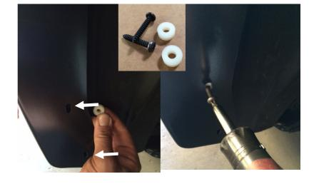
**STEP 6:** Slide the supplied spacers in behind the Fender Flare to fill the gap between the flare and the splash guard/fender. Use a screwdriver or the provided long screws to locate the spacers in line with the factory attachment points. Do not fully tighten screws at this stage.
