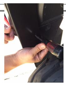
**STEP 15:** At the remaining open 3 slot positions in the Fender Flare, slide the spacer in behind the Fender Flare to fill the gap between the flare and the mud flap / splash guard.
