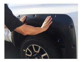
**STEP 18:** If necessary, make minor adjustments to the flare's position to achieve the best fit for your vehicle. When satisfied fully tighten all screw locations, in the above order on which they were installed, to ensure rubber seal is flush neatly against the body.
