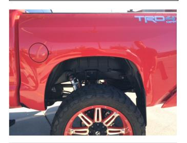
**STEP 10:** Clean the body area where the Fender Flares will make contact. Ensure fenders are dry prior to install.
