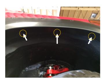
**STEP 7:** Locate the clips in the slots on the Fender Flare as shown.
