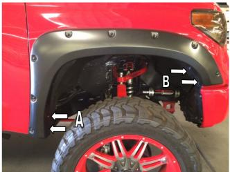
**STEP 1:** Clean the body areas where the Fender Flares will make contact. Ensure fenders are dry prior to install. Turn tires facing outward to provide additional room and ease hardware installation per side.
