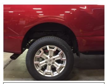
**STEP 8:** Clean the body area where the Fender Flares will make contact. Ensure fenders are dry prior to install. For models equipped with factory fender flares, removal of factory flares is required, please consult the vehicle service manual for factory fender flare removal.
