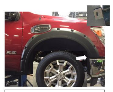
**STEP 7:** Install the provided U shape metal clip at the (1) remaining slot location in the Fender Flare. Ensure that positive pressure is applied on the Fender Flare to the vehicle fender when installing clips. Slide the clip over the Fender Flare and the inner lip of the front bumper fascia ensuring that the barb in the clip locates in the slot of the Fender Flare. Ensure that the rubber seal is flush neatly against the vehicle body.
