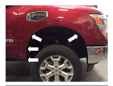
**STEP 5:** Place Fender Flare on the vehicle into the position of best fit. Note where (4) slots in Fender Flare correspond with (4) existing screws in the vehicle wheel arch molding. Remove Fender Flare. Remove the existing vehicle screws in locations as shown with #2 Phillips head screwdriver. Maintain screws for re-install.
