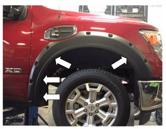
**STEP 6:** Place Fender Flare on vehicle, ensure the slots in the Fender Flare align with the holes in the wheel arch from the previously removed factory screws. Using #2 Phillips head screwdriver, re-install the previously removed (4) screws through slots in Fender Flare. Once positioned correctly ensure all fixing points are tight and secure.
