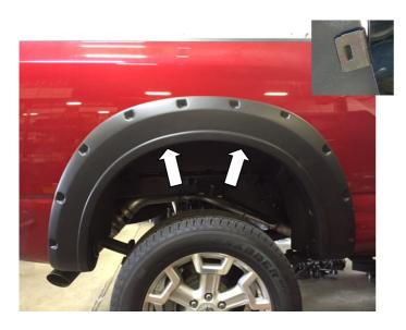
**STEP 12:** Install the provided U shape metal clips in the (2) remaining slot locations in the Fender Flare. Ensure that positive pressure is applied on the Fender Flare to the vehicle fender when installing clips. Slide the clip over the Fender Flare and the inner lip of the wheel arch ensuring that the barb in the clip locates in the slot of the Fender Flare. Ensure all fixing points are tight and secure and that the rubber seal is flush neatly against the vehicle body.
