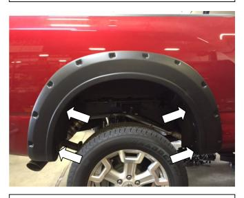
**STEP 11:** Place Fender Flare on vehicle, ensure the slots in the Fender Flare align with the holes in the wheel arch from the previously removed factory screws. Using #2 Phillips head screwdriver re-install the previously removed (4) screws through slots in Fender Flare. Once positioned correctly, ensure all fixing points are tight and secure.
