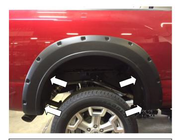
**STEP 10:** Place Fender Flare on the vehicle into the position of best fit. Note where (4) slots in Fender Flare correspond with (4) existing screws in the vehicle wheel arch. Remove Fender Flare. Remove only the existing vehicle screws in location as shown with a #2 Phillips head screwdriver. Maintain screws for re-install.
