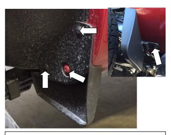
**STEP 9:** Using #2 Phillips head screwdriver, remove (4) screws from the forward factory splash guard deflector, (3) from inside wheel arch and (1) from the underside. Rear deflector will not work with Fender Flare instillation. Retain screws for fender flare install and store factory splash guard/deflector.
