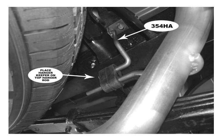
6) Place two of the supplied 2  $\frac{1}{2}$ " clamps **#MC250S** over the outlets of the muffler; then place right tailpipe **#16543** into position over the rear axle, and slide into the right muffler outlet. Connect the hanger that is welded to the rear of the pipe into the factory rubber hanger.
