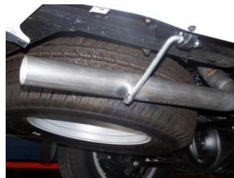
7. Install the exit pipe #D onto the tailpipe. Secure together with clamp #F. Do not tighten. Roll the exit pipe until it is at the correct angle for your vehicle. Insert welded hanger into rubber grommet.
