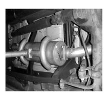
SLIDE MUFFLER #B WITH DUAL INLET ONTO HEADPIPE AT LEAST 1-1/2" TO 2". MUFFLER OUTLET SHOULD BE AT THE 12 O'CLOCK POSITION. USE CLAMPS #F TO ATTACH IT TO THE HEADPIPE. MAKE SURE INLETS AND MUFFLER IS LEVEL. USE JACK STAND TO SUPPORT MUFFLER. DO NOT TIGHTEN.
