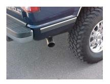
INSTALL TURNOUT PIPE #D INTO TAILPIPE USING CLAMP #G. INSTALL THE STAINLESS TIP. AND CLAMP DOWN. USE ANY STAINLESS STEEL OR ALUMINUM CLEANER TO POLISH TIP. DENALI & ESCALADE- YOU MAY NEED TO CUT 2" OFF THE REAR OF THE OVERAXLE PIPE SO THE TIP WILL BE CENTER WITH THE CUTOUT.
