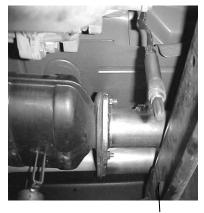
REMOVE O2 SENSOR FROM STOCK HEAD PIPE AND UNBOLT STOCK HEAD-PIPE.
