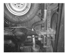
INSTALL THE OVERAXLE TAILPIPE #C INTO MUFFLER AT LEAST 1 1/2" TO 2" USING CLAMP #G. DO NOT TIGHTEN. INSERT WELDED HANGERS INTO RUBBER GROMMETS. THE SPARE TIRE ON SOME VEHICLES MAY NEED TO BE LOOSENED AND PULLED TO THE DRIVER SIDE AND RE-TIGHTENED. **ROTATE PIPES UNTIL YOU** HAVE AT LEAST A 1" CLEARANCE AWAY FROM ALL SHOCKS AND LEAF SPRINGS.
