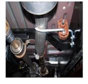
INSTALL HEADPIPE #A ONTO STOCK FLANGE. INSERT WELDED HANGER INTO RUBBER GROMMET. USE BOLT KIT PROVIDED TO SECURE. DO NOT TIGHTEN.
