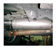
**INSTALL MUFFLER # B** ONTO HEADPIPE 1 ½" TO 2". USE CLAMP # F TO SECURE MUFFLER TO HEADPIPE. DO NOT TIGHTEN. USE A JACK STAND TO HOLD UP THE MUFFLER. OUTLETS SHOULD BE LEVEL.
