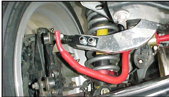
**IMPORTANT:** For proper maintenance grease the bushings at least once a year (15,000 miles) or whenever excessive noise occurs. Use a non-lithium based grease only! Lithium-based grease can wash out with water and should not be used.
