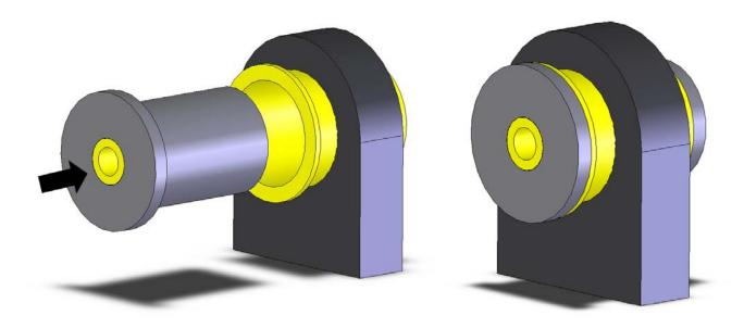
5. Install the thrust washer onto the unflanged side of the can.
