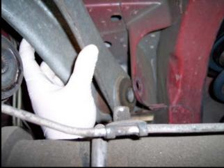
Now here comes the difficult part; removing the stock Can Bushings. These are the bushings that connect the aft end of the upper trailing arms to the differential.
