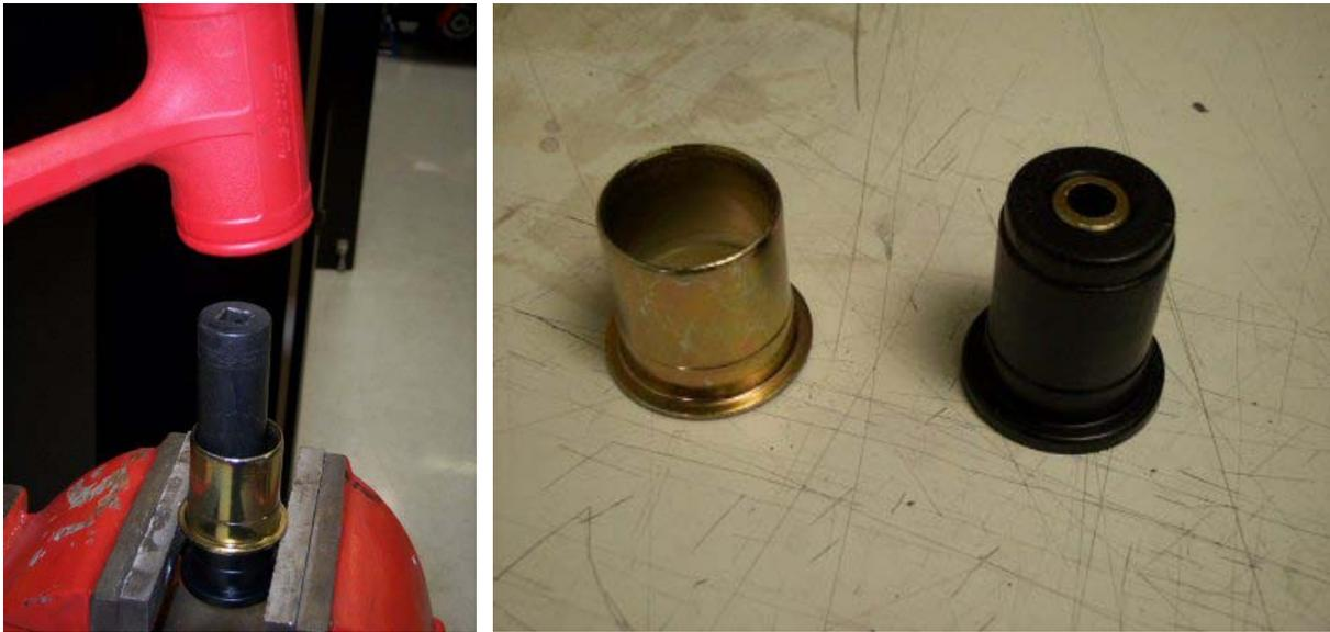
11. Normally with enough room, you can place the bushing can in the differential mount and hammer it in with a flat piece of wood. But, if there isn't enough room, then you will have to fabricate your own press tool. This is not as hard as it sounds.
