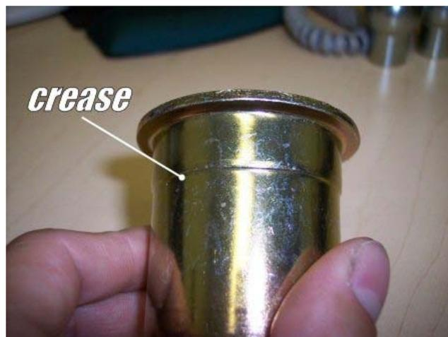
Important Note: On 12-bolt differentials, you cannot use the homemade press method. This is because the thrust bushing (see step 13) needs to be installed onto the can just before the can is fully pressed in. The thrust washer also needs to be shaved down in order to clear the differential housing. In this instance, use a dead blow hammer to smack the can into the mount hole.
