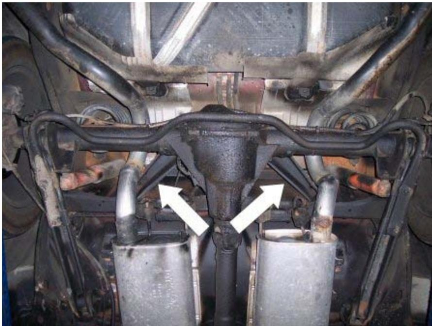
8. Now here comes the difficult part. Removing the stock Can Bushings. These are the bushings that connect the aft end of the upper trailing arms to the differential.
