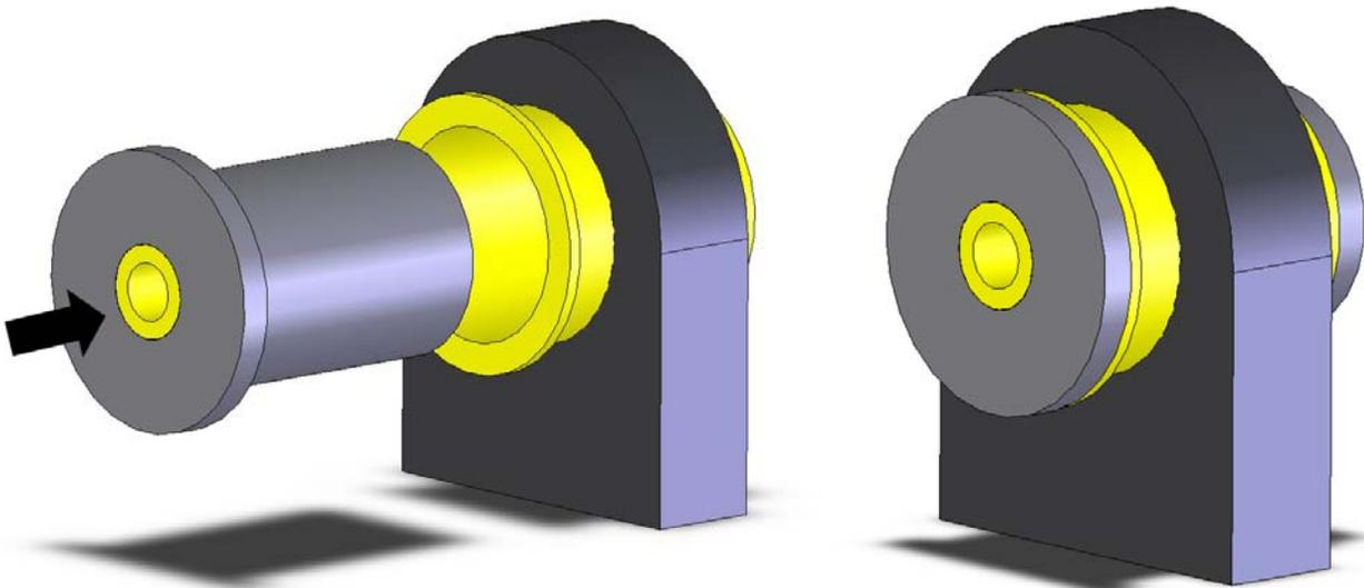
5. Install the thrust washer onto the unflanged side of the can.
