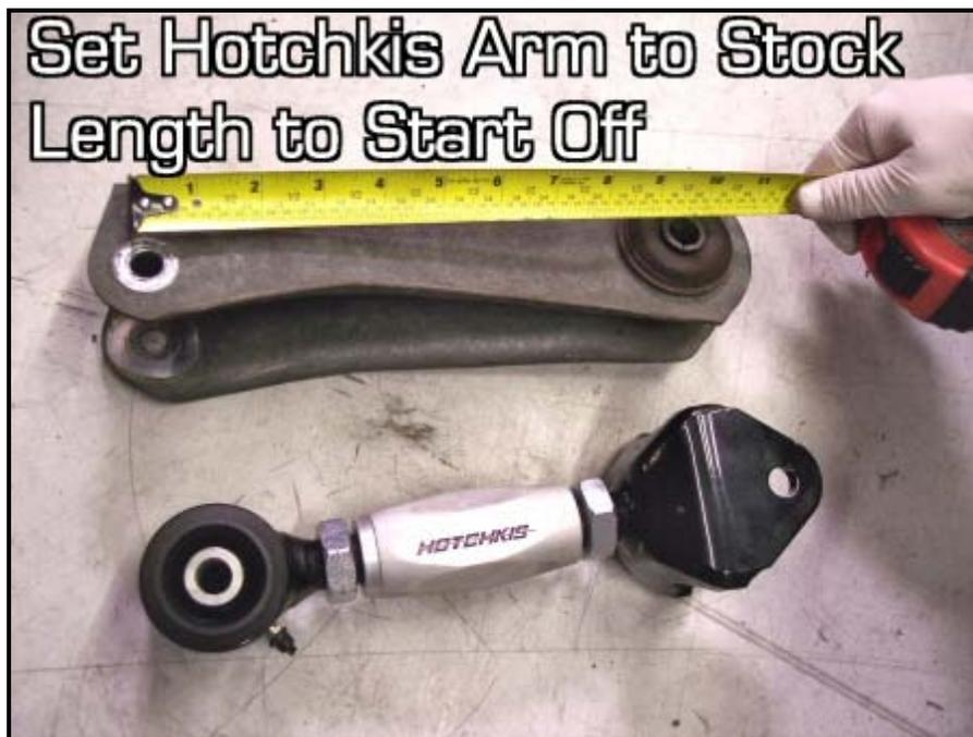
7. Install your new Hotchkis adjustable upper trailing arms in the same manner as the stock removal. Make sure the grease fittings on the front end are facing downward. Use all new hardware provided in your kit. Grease any polyurethane surface that contacts metal with the provided lube.
