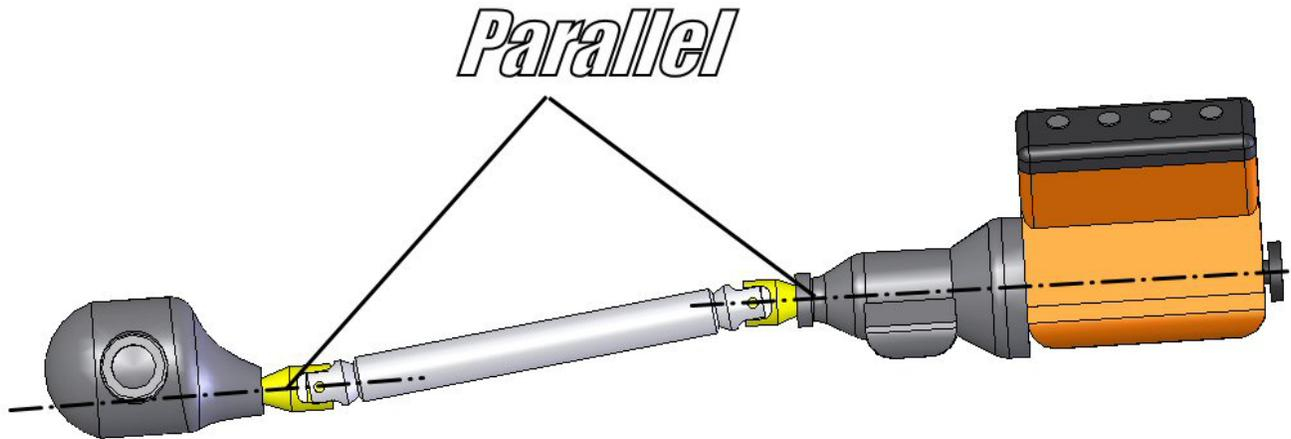
FYI... The centerlines should not be the same line because the U-joints would wear in the same areas all the time. Having an angle at the joint itself allows the joint to articulate and wear evenly along the entire bearing race.
