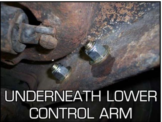
Reassemble the end links. Tighten the end links until you start to see the bushings begin to bulge.
