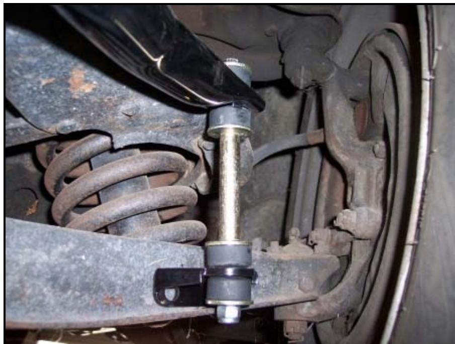
Mark the hole centers on the lower control arm with a marker. Once the holes are marked, you can disassemble the end links from the bar.
