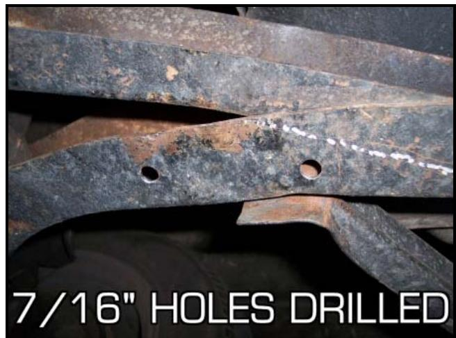
Once the holes are drilled out, undo the nut & bolt that holds the bumper support to the frame rail. This will give you enough clearance to install the reinforcement plate inside the frame rail. Install both reinforcement plates and re-install the bumper support nut & bolt.
