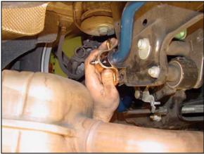
9/ Re-install the end link bolts (using the supplied 10mm washers in between the nut and the end link head) and nuts and leave loose. Secure the bushing brackets, using the supplied 8mm washers in between the nuts and the slots of the bushing brackets. Tighten the four bracket bolts, then tighten the end link bolts.
