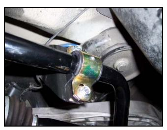
Attach the end links to the bar ends (inner hole for more roll resistance and the outer hole {near the ends} for less roll resistance) using the 10mm bolts, nylock nuts and small and large washer. Use the large diameter washer to capture the outboard side of the end link bushing and the smaller washer for the inboard side against the sway bar end.
