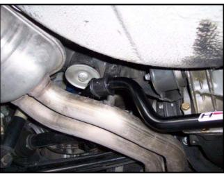
10) Next, slide the bushing brackets over the bushings. Position the bracket onto the stock mounting point. Fasten the bushing bracket using the provided 8mmx20mm bolt and washer.
