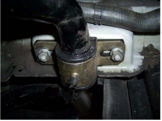
5) Apply grease along the inside surface of your polyurethane bushings and attach them to the H-Sport bar in the approximate mounting locations. Slip the new brackets over the bushings.
