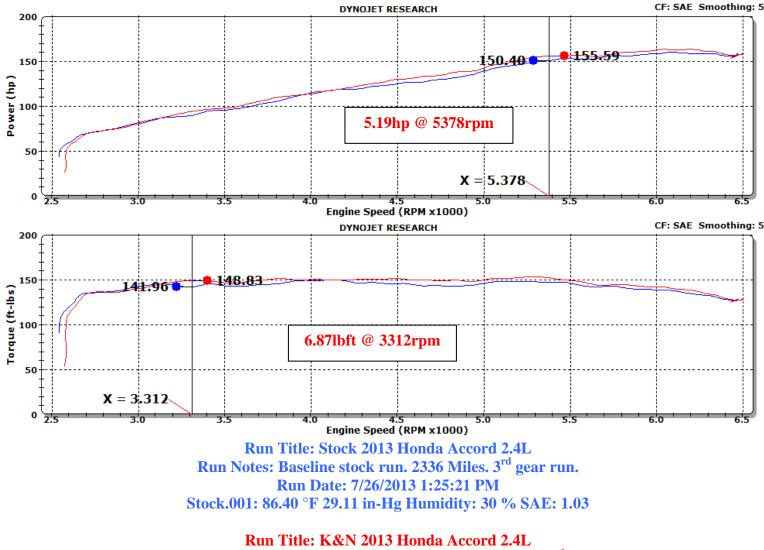
Run Notes: K&N intake kit #69-1213 installed. 2336 miles. 3<sup>rd</sup> gear run. Run Date: 7/26/2013 1:25:21 PM K&N.002: 86.40 °F 29.11 in-Hg Humidity: 30 % SAE: 1.03
