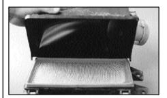
Unclip the two retaining clips and remove stock filter.
