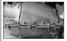
Line up the hinges, close the airbox and secure it with the spring clips.
