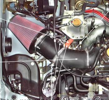
**3.** Fit the MAS into the new intake hose, reconnect the electrical harness plug to the MAS (If necessary rotate the MAS slightly to ensure the harness / plug clears the coolant reservoir. Secure the MAS with the #60 studded clip. Attach the clip to the mounting bracket using a nut and washer supplied. Fully tighten all the hose clips.
