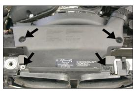
3. Pull up on the four fresh air duct-retaining pins to release them from the radiator core support.
