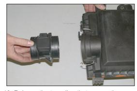
19. Release the two clips that secure the mass air sensor to the air box, then remove the mass air sensor as shown.
