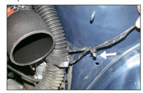
21. Using a pair of pliers, carefully remove the wiring harness retaining clip from the inner fender as shown.
