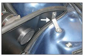
26. Install the provided bracket onto the heat shield and inner fender with the provided hardware as shown.
