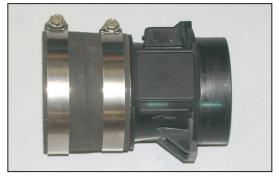
20. Install the silicone hose (08690) onto the mass air sensor and secure with the provided hose clamp.
