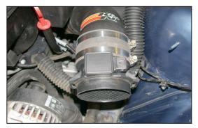
22. Install the mass air sensor assembly onto the  $K\&N^{\circledcirc}$  intake tube and secure with the provided hose clamp.
