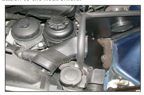
27. Install the factory fresh air tube into the heat shield as shown.
