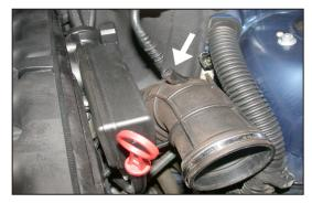
9. Disconnect the vent tube from the factory intake tube as shown.
