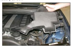
8. Lift up and remove the air box from the vehicle. NOTE: K&N Engineering, Inc., recommends that customers do not discard factory air intake.
