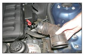
10. Loosen the lower hose clamp and remove the factory upper intake hose from the lower intake hose.
