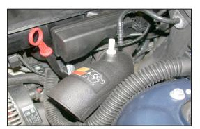
13. Install the K&N<sup>®</sup> intake tube into the factory lower intake hose and secure with the factory hose clamp.
