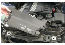
4. Lift up and remove the fresh air duct from the vehicle as shown.
