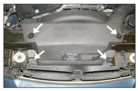
28. Reinstall the fresh air duct removed in step #4 and secure with the four factory retaining pins.
