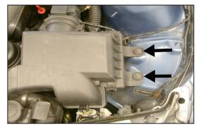
6. Remove the two factory air box mounting bolts shown.
