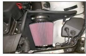
24. Install the K&N® air filter onto the K&N® intake tube and secure with the provided hose clamp.
