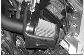
20. Install the K&N® Filtercharger onto the K&N® intake tube and secure it with the provided hose
