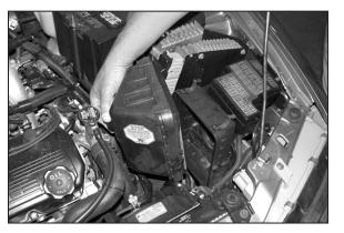
4. Unclip the four over-center clamps on the air cleaner, then remove the air cleaner lid as shown
