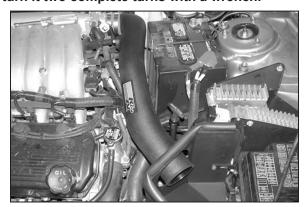
16. Install the K&N® intake tube into the hole on the heat shield, then slide the other end into the silicone hose at the throttle body.
