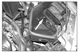
12. Install the heat shield assembly and line up the "L" bracket with the original air cleaner mounting point, then, line up the angled bracket with the mounting point on the electric fan and secure with the provide hardware.
