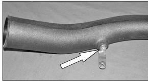
14. Install the Angled "L" bracket onto the K&N® intake tube and secure with the provided hardware.
