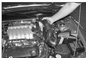
3. Loosen the hose clamps at the throttle body and at the air cleaner assembly, then remove the stock intake tube as shown
