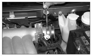
13. Install the provided silicone hose and hose clamps onto the throttle body as shown.
