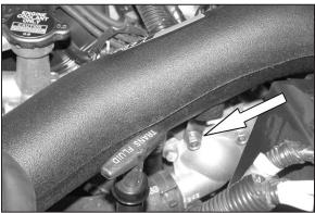
17. Using the bolt removed in step 7, secure the angled "L" bracket to the water neck as shown.
