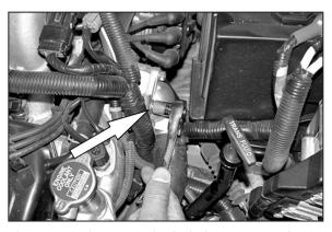
7. Loosen and remove the bolt that secures the wire harness bracket to the water neck as shown.
