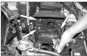
5. Loosen and remove the three bolts that secure the air cleaner base to the inner fender as shown.
