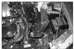
6. Using a flat blade screwdriver depress the tabs on the air inlet to release the air cleaner base, then remove the air cleaner base as shown.
