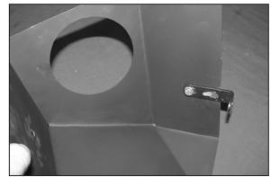
9. Secure the "L" bracket to the heat shield using the provided hardware as shown.
