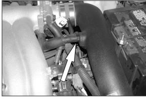
19. Reconnect the crank case vent hose to the vent on the K&N® intake tube as shown.
