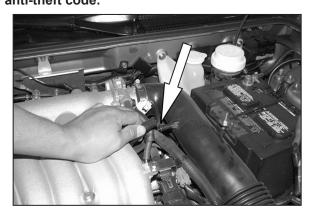
2. Disconnect the crank case vent hose from the stock intake tube as shown
