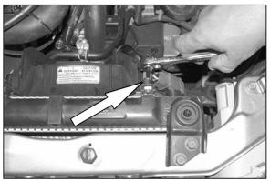
8. Loosen and remove the bolt that secures the electric fan to the radiator as shown.
