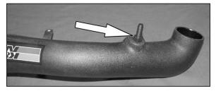
15. Install the provided vent into the threaded vent on the K&N® intake tube as shown.
