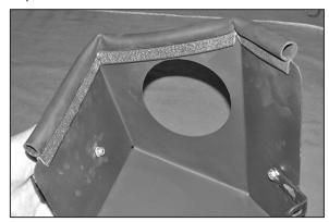
11. Apply the provided trim seal to the heat shield assembly as shown.
