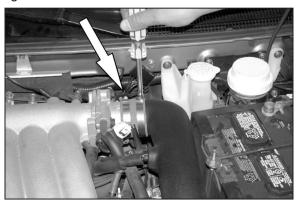
18. Tighten the hose clamp on the K&N® intake tube as shown.
