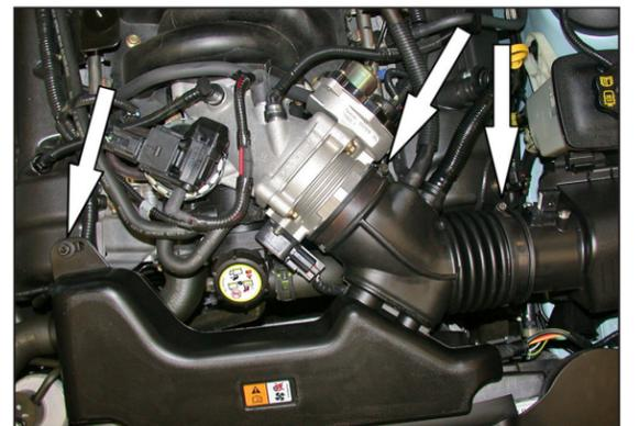
7. Loosen the hose clamps at the throttle body and the factory air box, and then remove the intake tube retaining nut shown.
