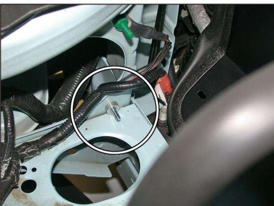
14. Install the provided 6mm bolt through the factory hole in the core support and then install the provided spacer onto the bolt as shown.
