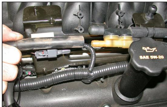
5. Disconnect the evaporative hose from the evaporative valve and cut the two tie wraps securing the hose to the bracket.
