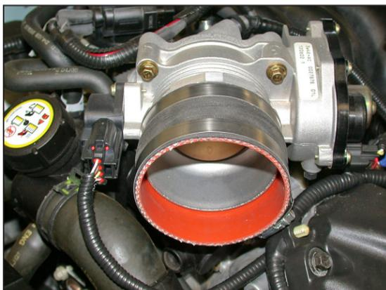
18. Install the provided silicone hose (08630) onto the throttle body and secure with the provided hose clamp.
