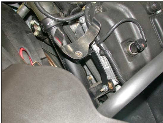
17. Install the saddle bracket assembly onto the threaded stud on the engine as shown and secure with the provided hardware.
