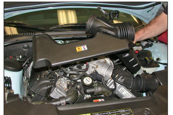
8. Remove the stock intake tube assembly from the vehicle.
