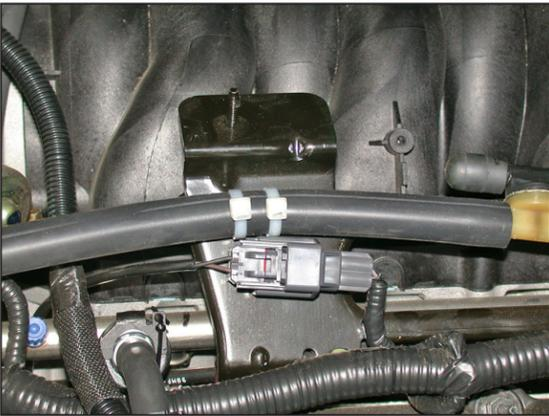
28. Using the two supplied tie wraps, secure the evaporative hose retaining clip as shown.
