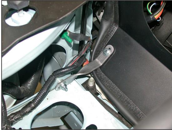
15. Install the provided heat shield bracket (010084) onto the bolt installed in step #14, and then fasten the bracket to the heat shield with the provided hardware.
