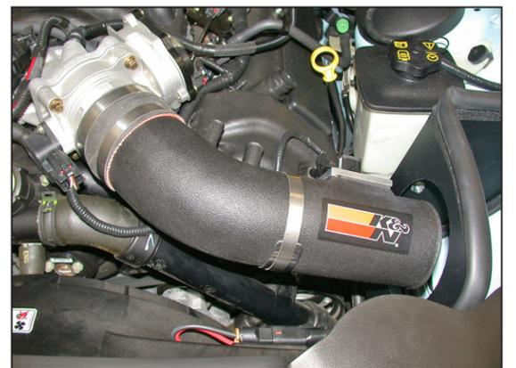
23. Install the K&N® intake tube assembly into the silicone hose at the throttle body and onto the saddle clamp and secure with the provided hose clamp as shown.
