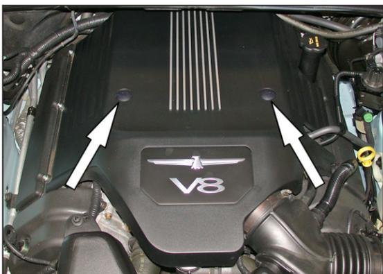
2. Remove the two plastic screws shown securing the engine cover.
