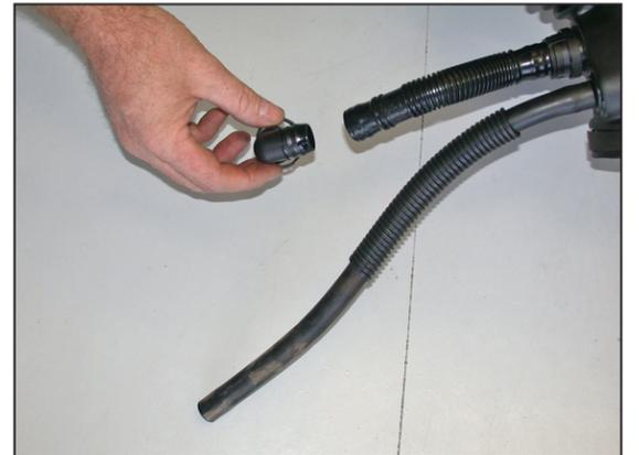
24. Pull firmly on the crank case vent elbow to remove from the vent tube as shown.
