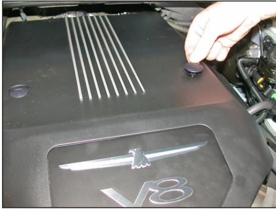
31. Reinstall the engine cover onto the rear retaining clips and then reinstall the retaining clips removed in step #2.
