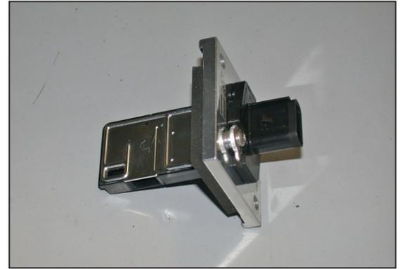
21. Using the screws removed in step #19, install the mass air sensor into the K&N® mass air adapter.
