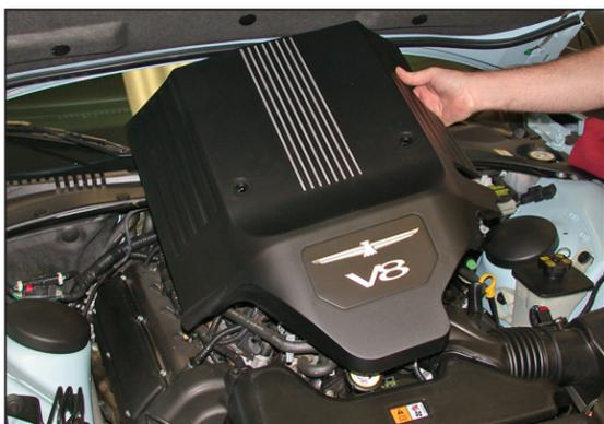
3. Pull up on the rear of the engine cover to dislodge from the retaining mounts, and then remove the engine cover from the engine.
