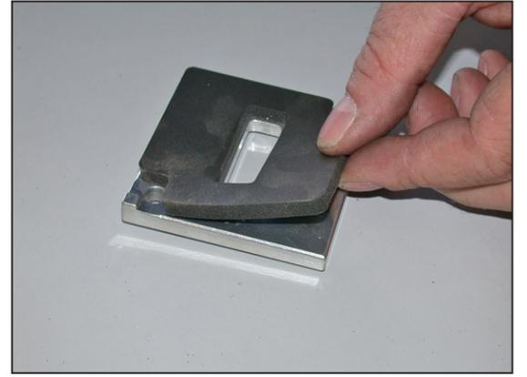
20. Install the provided gasket onto the K&N® mass air adapter as shown.
