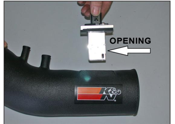
22. Install the mass air assembly into the K&N® intake tube and secure with the provided hardware.
