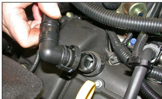
6. Depress the locking ring on the crank case vent hose, and then remove the crank case vent hose from the valve cover.
