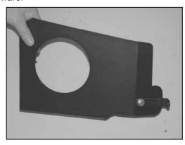
12. Install the "L" bracket (07158) onto the front of the heat shield as shown with the provided hardware.
