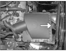
5. Remove the air box mounting bolt shown.
