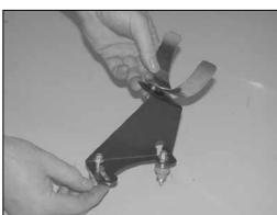
9. Install the valve cover bolts removed in step #8 into the tube mounting bracket as shown passing through the key hole portion and then slide the bolts to the end of the slots.
