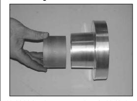
22. Vehicles that come equipped with Hydracarbon trap, place the Hydrocarbon trap into the filter adapter as shown.
