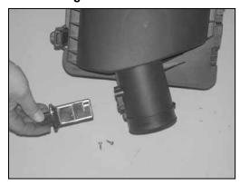
16. Remove the mass air sensor from the factory air box with the T20 "TORX" wrench provided.
