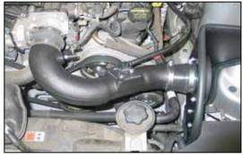
22. Install the intake tube into the silicone hose at the filter adapter and then into the hump hose at the throttle body and then secure with the provided hose clamps.
