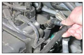
23. Remove the crank case vent tube assembly from the valve cover port.
