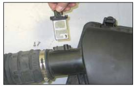
19. Remove the two screws which secure the mass air sensor and then remove the mass air sensor from the stock air box.
