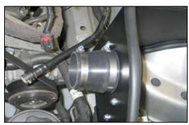
16. Install the provided step hose (084055) onto the filter adapter and secure with the provided hose clamp.
