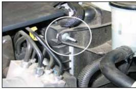
13. Remove the fan shroud mounting bolt shown.
