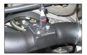
28. Connect the provided mass air sensor extension harness into the factory harness and then connect the open end into the mass air sensor.
