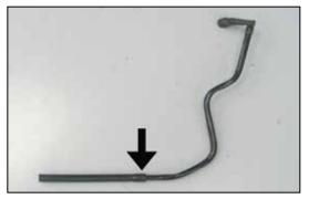
25. Install the 9" section of silicone hose provided onto the cut factory crank case vent tube as shown.
