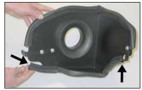
12. Install the shorter 20" section of edge trim onto the heat shield as shown.
