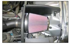
27. Install the K&N<sup>®</sup> air filter and secure with the provided hose clamp.
