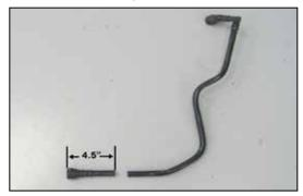
24. Cut the crank case vent tube as shown 4.5" from the end which attaches to the intake tube.
