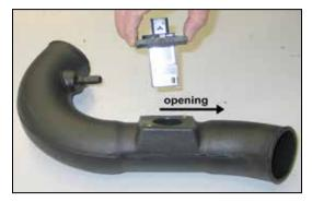
21. Install mass air sensor assembly into the intake tube and secure with the provided hardware. NOTE: Be sure to install the sensor with the opening pointed towards the filter end of the intake tube. end to the npt fitting installed into the intake tube. NOTE: It will be necessary to trim the silicone vent hose.
