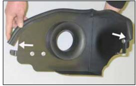
11. Install the longer 27" section of edge trim onto the heat shield as shown.
