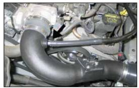
26. Reinstall the crank case vent hose assembly onto the valve cover and then connect the open and to the intelled into the intelled type.
