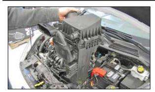
7. Remove the complete air box assembly from the vehicle by pulling up to release it from the grommets.
