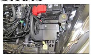
11. Install the heat shield into the vehicle so that the two mounting posts engage the air box mounting grommets.
