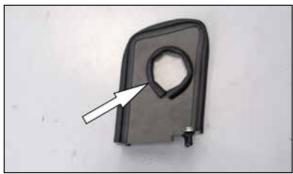
10. Install the provided "Side Bulb" edge trim around the inside of the hole in the heat shield as shown.
