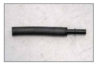
22. Install the provided EVAP vent hose onto the provided quick disconnect union as shown.
