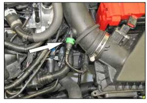
4. Release the green locking tab and then disconnect the EVAP vent line from the factory intake tube.
