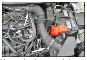
5. Loosen the hose clamps securing the factory intake tube to the turbo inlet pipe and to the factory air filter housing. Remove the factory intake tube from the vehicle.
