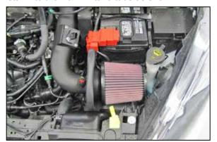
24. Install the K&N® air filter onto the intake tube and secure with the provided hose clamp.
