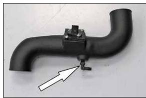
20. Install the 90° vent fitting into the K&N® intake tube as shown.
