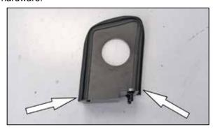
9.Install the provided "Top Bulb" edge trim around the outside of the heat shield as shown.
