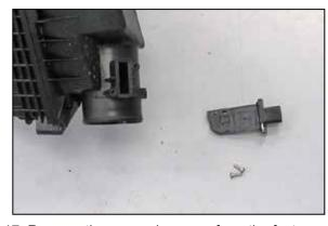
17. Remove the mass air sensor from the factory air box.
