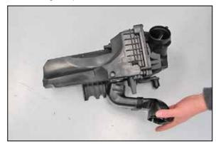
13. Remove the fresh air intake duct from the factory air box by pulling it away.
