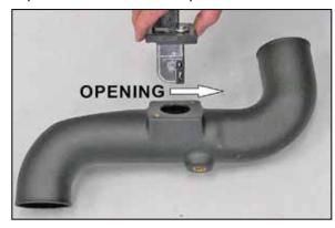
19. Install the mass air sensor assembly into the K&N intake tube and secure with the provided hardware.
